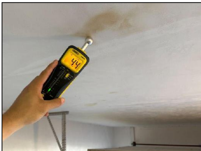
36. Stains on ceiling. NO moisture detected...
